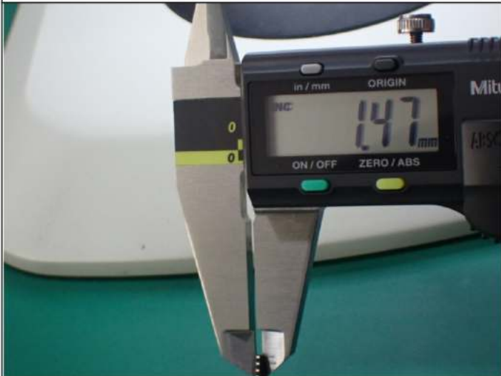
Parts as arrived: C=1.47mm (PASS)
