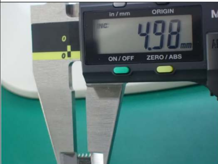
Parts as arrived: A=4.98mm (PASS)
